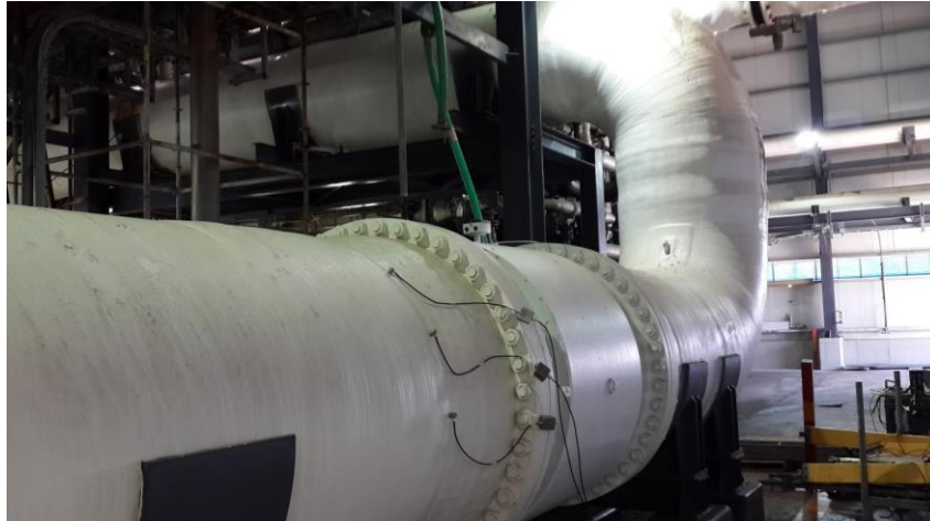
Acoustic Emission monitoring of FRP piping
