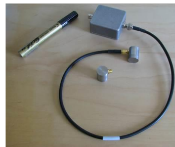
AE sensors and preamplifier
